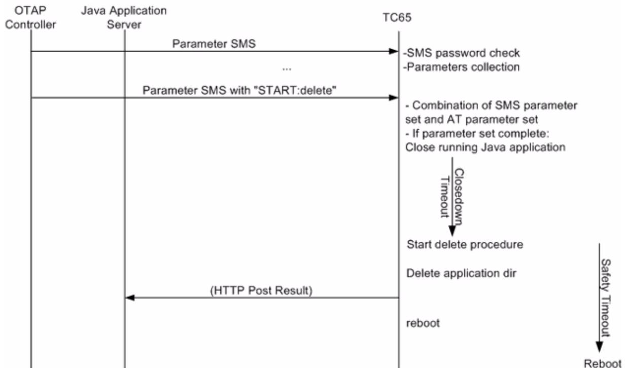
Figure 21: OTAP: Delete Information Flow (messages in brackets are optional)
