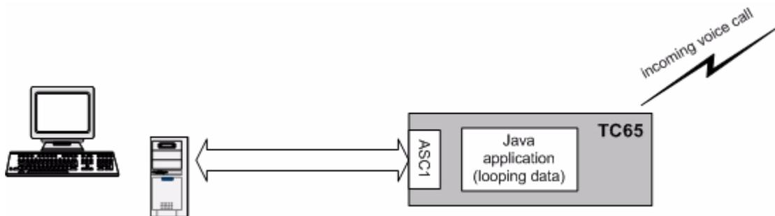
Figure 16: Scenario for testing data rates on ASC1 with a voice call in parallel
