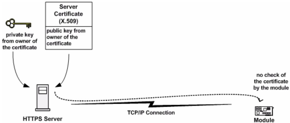
Figure 59: Mode 1 – Customer Root Certificate does not exist
