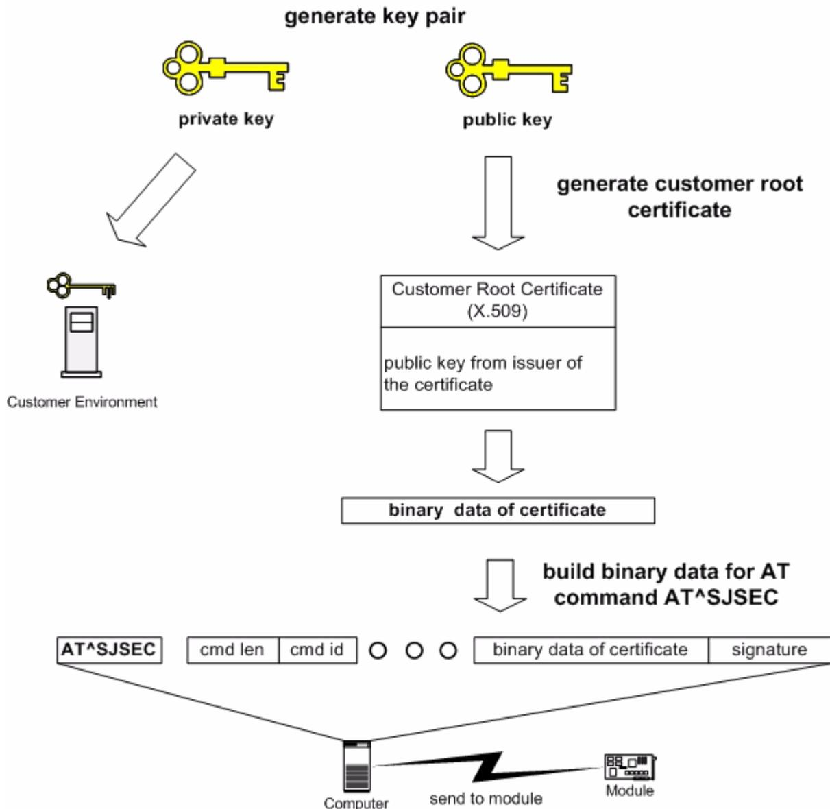
**Figure 62:** Insert Customer Root Certificate
