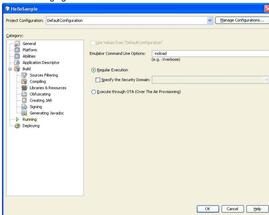
**Figure 36:** NetBeans IDE 6.0.1 - add emulator option “-noload” (e.g. project “HelloSample”)
